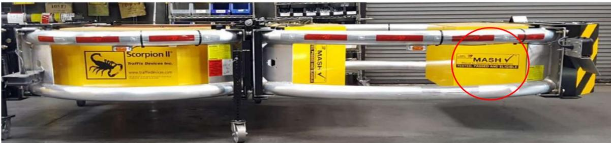
The STMS should always do an equipment check before leaving the yard. This includes all electronic displays and TMAs. Even slight damage can considerably degrade the performance of the TMA.
